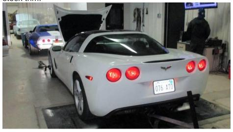
Dynometer results for a stock trim 2008 C6 Coupe equipped with an automatic transmission show 370.8 RWHP (rear wheel horsepower) at approximately
