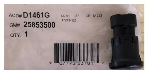
Any C6 owners having problems opening the rear hatch on either a coup or convertible, it's generally the button down by the license plate that is at fault. The button (GM part number 25853500) costs about \$15. To replace it, you take out the passenger side inboard taillight, reach in and pinch in the two tabs holding the switch in place. Pull the switch down and disconnect electrical connector. Install the new switch in reverse sequence.
